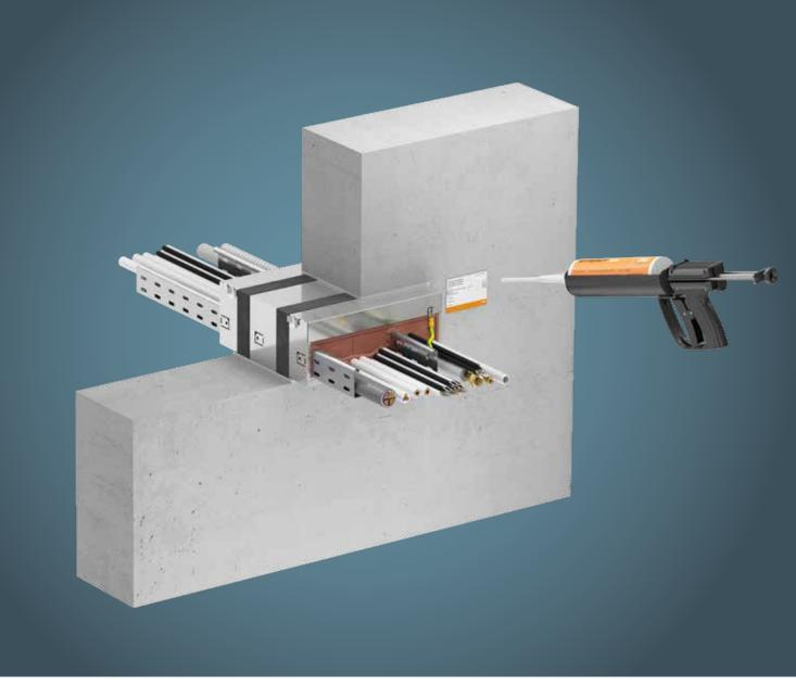
The new 4-sided variant of the OBO fire protection box consists of a two-part stainless steel housing with intumescent fire protection inlays. It can be used as an insulation system in walls and ceilings. Their releasable Magic connection means they are very quick to mount. Simply click the halves of the housing together, insert them in the component opening and mortar them in. Side straps secure the correct position of the PYROPLUG<sup>®</sup> MagicBox, allowing safe mortaring.
