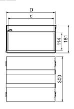
PYROPLUG® MagicBox, four-sided, interior height 110 mm
