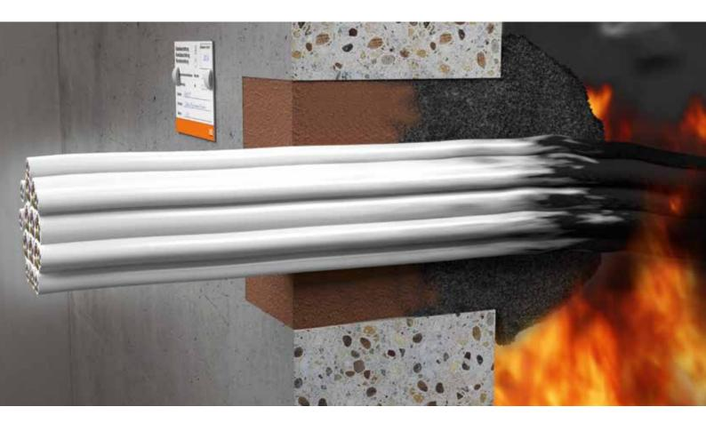
Electrical cables and pipes may only be run through walls and ceilings at the ends of rooms when there is a guarantee that they do not present an opportunity for fire and smoke to spread. Set against this background, the installations required for ceiling and wall penetrations must be reliably sealed. This is done using insulation systems, which effectively prevent the spread of fire and smoke.
