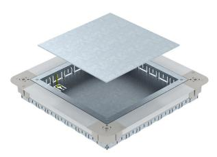
Underfloor accessory box with mounting lid and lid blanking plate with sheet steel side walls. For the installation of a square GES9 55 service outlet in screed heights of 55 mm or more. Height can be infinitely adjusted to the nominal screed height and the screed can be worked flush to the screed scraping edge. With 7 x M20, 3 x M25, 4 x M32 pipe insertion openings on each side. Usable pipe size at a system height of 55 mm: M20.
