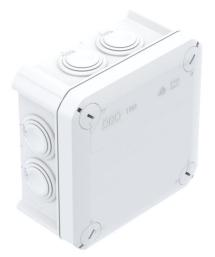
Junction box for the connection of cables and lines indoors and in protected outdoor areas. Square design with plug-in seals to the sides and knock-out entries in the bottom. Suitable for wall and ceiling mounting and on mounting panels. With the option to fasten inside and to mount via the corner domes. Cover with quick lock, sealable. Made from halogen-free and UV-resistant materials.
