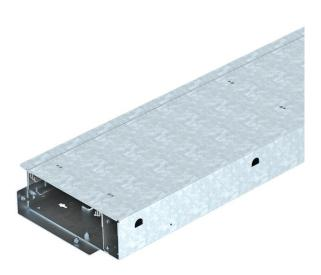
Ready-to-mount trunking unit for cable routing and device installation, consisting of a trunking base with two blanking covers. The scope of delivery contains two lid butt seals and one connector. For height adjustment, six height adjustment units are required. Load capacity up to a maximum of 5 kN. The trunking unit can be supplemented with an adjustable floor covering contact profile for screed limitation in areas of door frames and in front of radiator niches.
