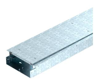
Ready-to-mount trunking unit for cable routing, consisting of a trunking base with two covers. The scope of delivery contains two lid butt seals and one connector. For height adjustment, six height adjustment units are required. Load capacity up to a maximum of 5 kN. The trunking unit can be supplemented with an adjustable floor covering contact profile for screed limitation in areas of door frames and in front of radiator niches.
