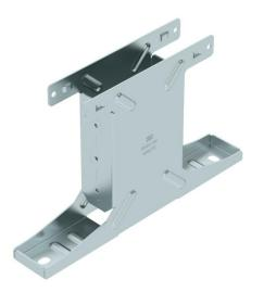
Base of the symmetrical floor support for the BKRS system, suitable for crossbeam type BSST 400/500/600. Can be used for walkable cable trays of width 400-600 mm. With threaded unions for mounting connection components, e.g. pipe clamps, as well as slots for floor mounting up to M10. Fastening material must be ordered separately.
