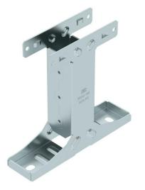
Base of the symmetrical floor support for the BKRS system, suitable for crossbeam type BSST 200/300. Can be used for walkable cable trays of width 200 or 300 mm. With threaded unions for mounting connection components, e.g. pipe clamps, as well as slots for floor mounting up to M10. Fastening material must be ordered separately.
