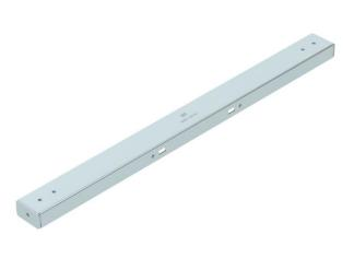
Crossbeam of the symmetrical floor support for the BKRS system, suitable for base type BSSU 190 4060. Can be used for walkable cable trays of width 600 mm. With threaded unions for cut-free mounting of cable trays. Fastening to base with 4x FKS M6 flat-head screws. Fastening material must be ordered separately.
