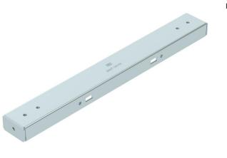
Crossbeam of the symmetrical floor support for the BKRS system, suitable for base type BSSU 190 4060. Can be used for walkable cable trays of width 400 mm. With threaded unions for cut-free mounting of cable trays. Fastening to base with 4x FKS M6 flat-head screws. Fastening material must be ordered separately.
