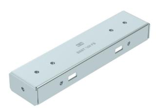
Crossbeam of the symmetrical floor support for the BKRS system, suitable for base type BSSU 190 2030. Can be used for walkable cable trays of width 200 mm. With threaded unions for cut-free mounting of cable trays. Fastening to base with 4x FKS M6 flat-head screws. Fastening material must be ordered separately.
