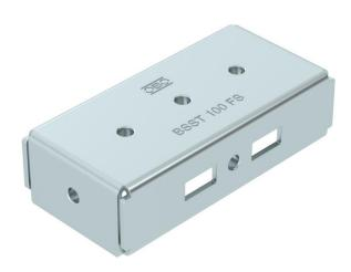
Crossbeam of the symmetrical floor support for the BKRS system, suitable for base type BSSU 190 1010. Can be used for walkable cable trays of width 100 mm. With threaded unions for cut-free mounting of cable trays. Fastening to base with 4x FKS M6 flat-head screws. Fastening material must be ordered separately.
